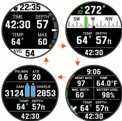
**Dive stopwatch:** Displays the bottom time stopwatch; current, maximum, and average depth; and rate of ascent or decent ([Using the Dive Stopwatch, page 8](#)).
