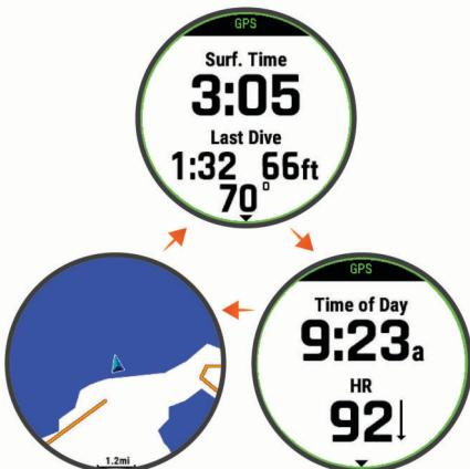
**Surface interval screen:** Displays the current surface interval time, as well as the elapsed time, maximum depth, and temperature for your last apnea dive.
