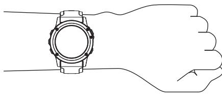
**NOTE:** While diving, the device should stay in contact with your skin, and it should not bump into other wrist-worn devices.
